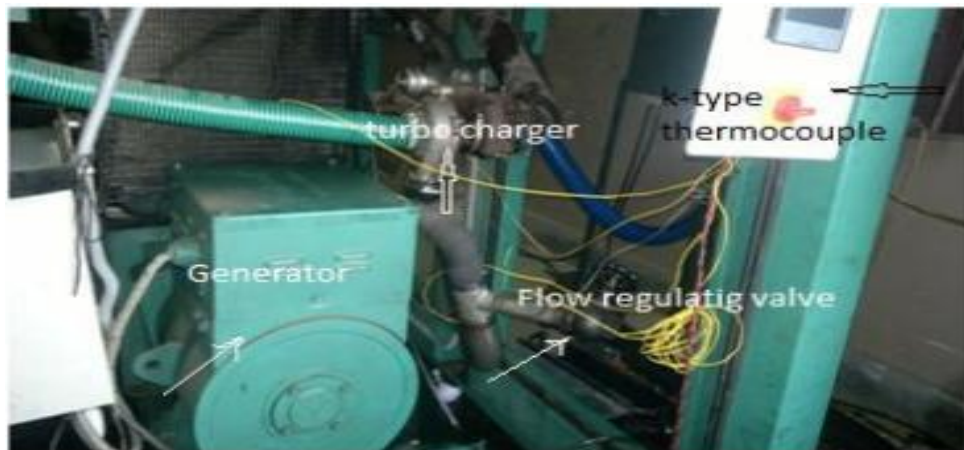
Fig. 1. Photographic view of engine setup under turbo mode operation
